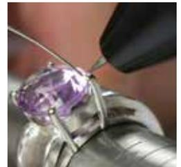
Re-tipping prongs is incredibly fast and easy using an Orion welder.
