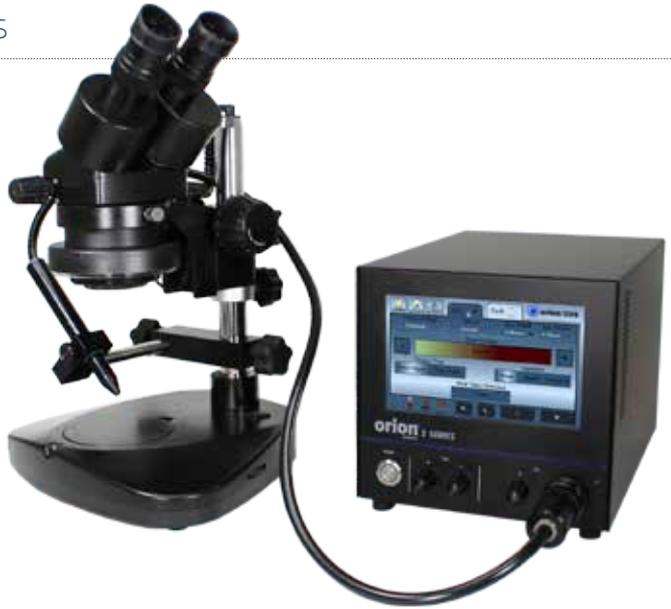
The Orion 150s is the perfect welder for those needing a wide range of power (from 1 – 150 joules of energy) to get work done. This mid-range solution includes a high-frequency agitation feature that adds deeper penetration and weld strength. The 150s, used on jewelers' benches around the world, surpasses any competing product in feature and price. When you need a straightforward welding solution, this is the machine you want.
